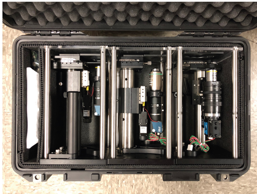
Supplementary Figure 5. Three Squid microscopes in a Pelican Air 1535 carry-on case.
